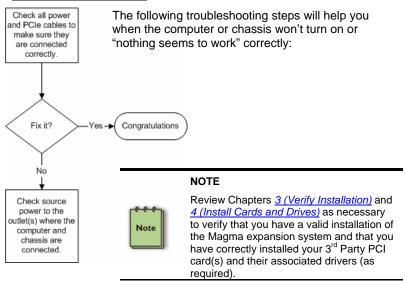
If it powers up OK, but nothing works, check the computer's Device Manager or System Profiler to see if the expansion system has been found. If not found, try the troubleshooting steps for My Computer Can't Find the PCI Expansion System. If the expansion system is visible, but has a problem, try to resolve the problem (See Note above). If that fails, go to Chapter 7 to see about getting additional help.
